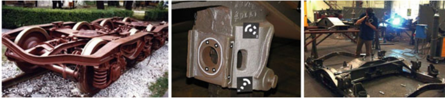
Fig. 12.17 Finished swivel-truck (left), a frame detail with the reference points and marked features (middle), the measuring process (right) [24]
