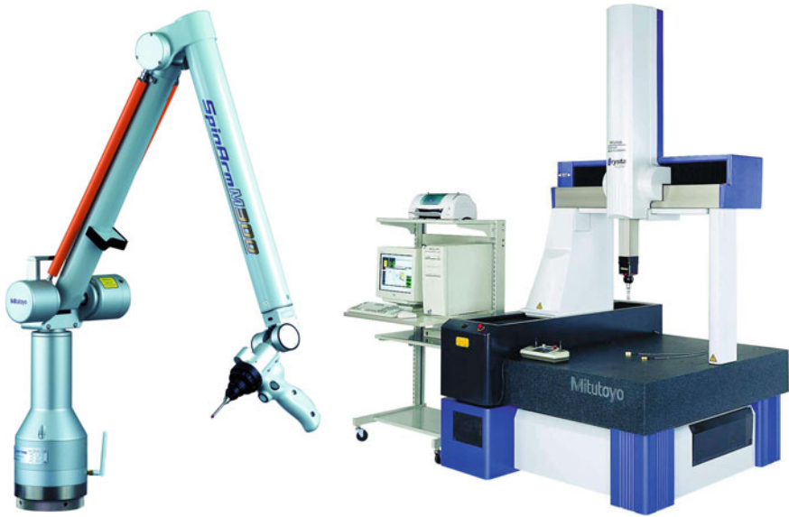
Fig. 12.6 Multi-axis tactile measurement machines: Spin Arm M, 7-axis articulated measurement arm and Crysta Apex, 3-axis CNC CMM (both from Mitutoyo)
