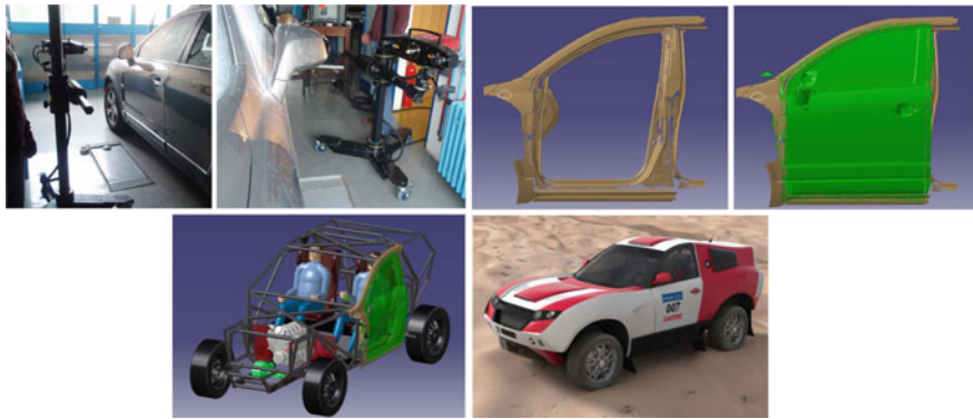
Fig. 12.15 The ATOS measurement (above, left), the 3D models made up of the STL files (above, right), a 3D model of the racing vehicle for the Croatian Dakar Rally Team (down) [23]
