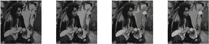
Fig. 8. Segmentation with 2, 3, 4, 5 thresholds for Barbara by PSO
