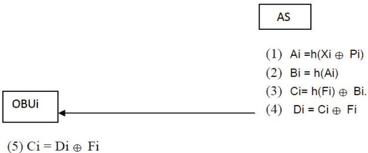
Fig. 2. Key Generation Procedure
