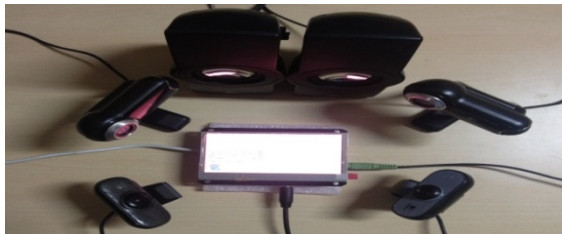
Fig. 5. Hardware for the lane departure detection system
