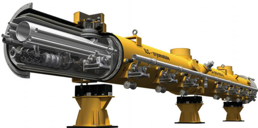
Fig. 8.11 A cut-view of the cross-section of ILC cryomodule. Cavity and other components are seen in the picture (© Rey.Hori/KEK)
