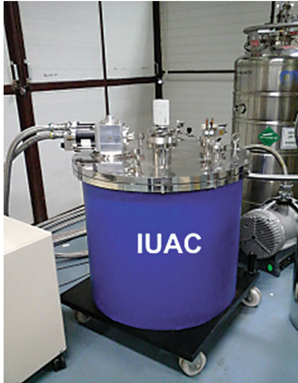
Fig. 7.28 The photograph of the complete CFMS system with central RT bore and all feed-thrus (Courtesy IUAC Delhi)
