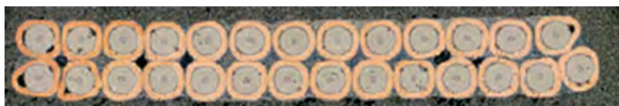
Fig. 6.40 A typical cross-section of a 27 strand Rutherford cable fabricated by a number of institutions in US and Japan
