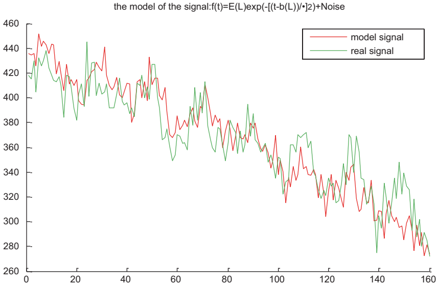
Fig. 108.6 The model of the signal f(t) = E(L)e^{-\left[\frac{(t-b(L))}{\tau}\right]^2} + \text{Noise}
