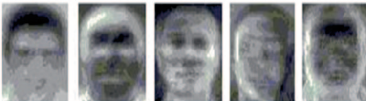
Fig. 111.2 The top five eigenfaces in ORL database
