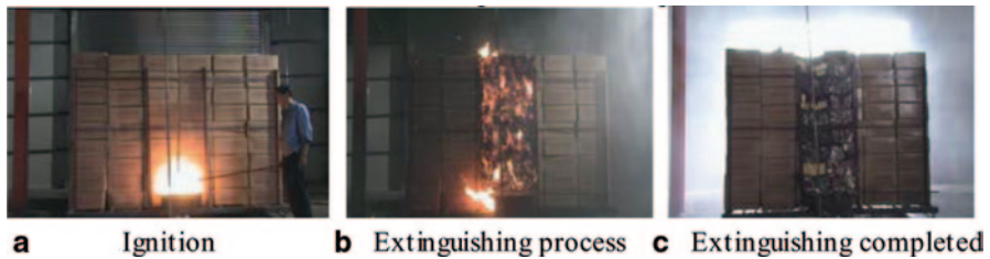
Fig. 133.4 Figure simulation single warehouse fire. a Ignition. b Extinguishing process. c Extinguishing completed
