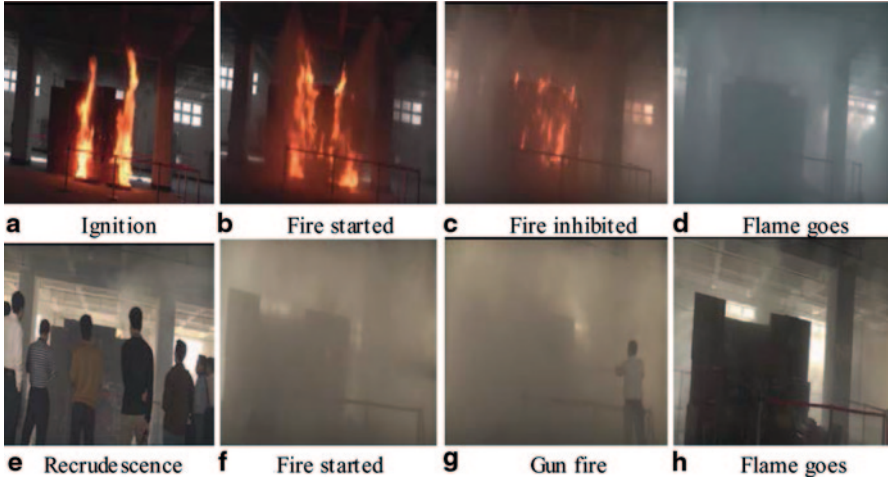
Fig. 133.6 Shi ma tobacco warehouse fire process diagram. a Ignition. b Fire started. c Fire inhibited. d Flame goes. e Recrudescence. f Fire started. g Gun fire. h Flame goes
