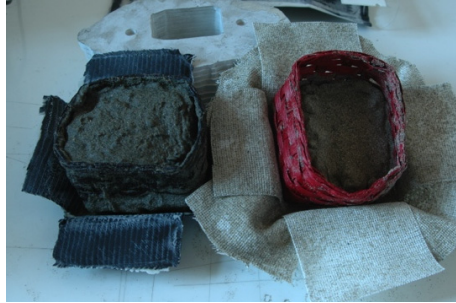
Fig. 3. Test in ISCR laboratory. On the right a basket recovered with 3M™ Scotchcast™ Plus Casting Tape; on the left a basket recovered with sheets of carbon fibre in a plastic bag vacuum. Photo ISCR –MBACT.
