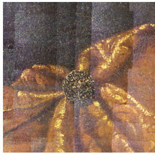
Fig. 2. Fragment of a painting composed from 36 directional measurements without any lighting non-uniformity correction
