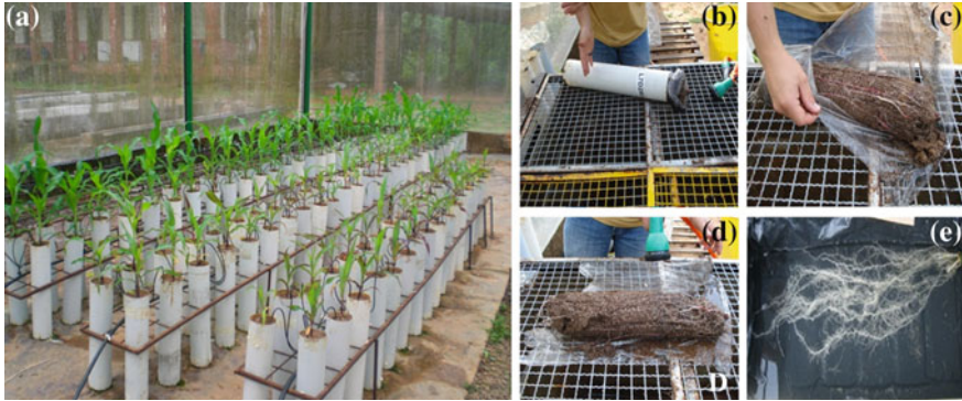
Fig. 4.1 Planting of maize strains in PVC pipes wrapped in plastic bags under high and low nitrogen availability (a); root washing process (b, c, and d); and the root system obtained using this technique (e)
