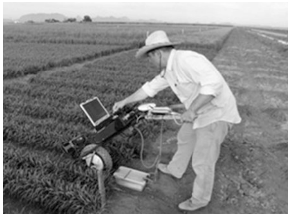
Fig. 6.4 This figure depicts a researcher using GPR to measure wheat root biomass (Thompson et al. 2013; used with permission)
