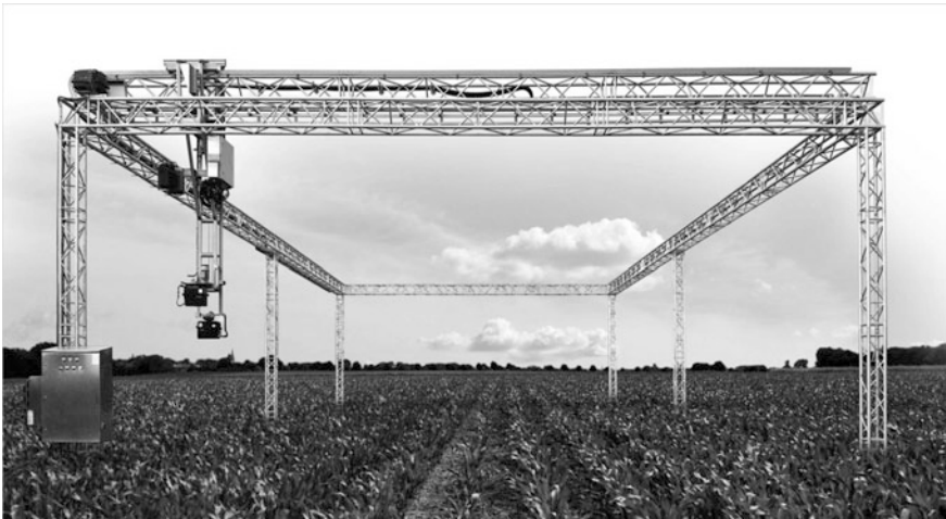
Fig. 6.5 The Lemnatech Scanalyzer Field platform for field-based phenotyping (Schwartz et al. 2013; used with permission.)
