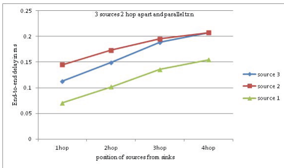
Fig. 10. End-to-end delay when three sources send to three sinks at a time in ms
