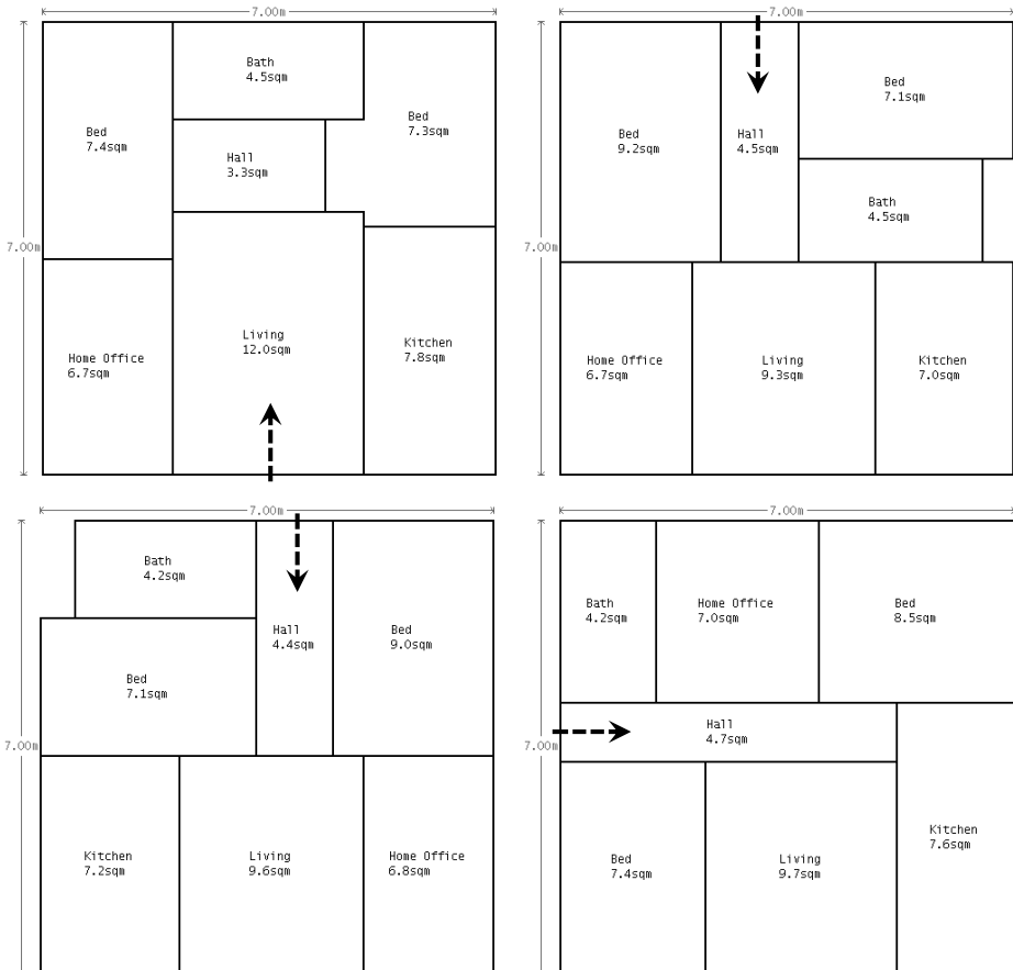
Fig. 3. Four usable solutions returned in one run for the apartment problem. Principal access is through the hall, or directly into the living room.
