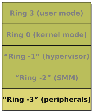
Fig. 2.1 “Ring -3” environment compared to other rootkit environments on the x86 platform. Please note, ring 3 and ring 0 are implemented in hardware (host CPU). The terms “ring -1”, “ring -2”, and “ring -3” are used to emphasize the power of the corresponding execution environments. They are not implemented in hardware
