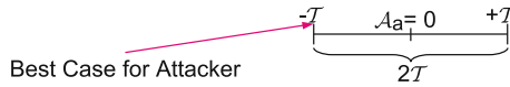
Fig. 5.5 Tolerance value \mathcal{T} . If the attacker can predict the very exact moment where BARM determines \mathcal{T} too little bus transactions, an attack with 2\mathcal{T} bus transactions could theoretically executed stealthily
