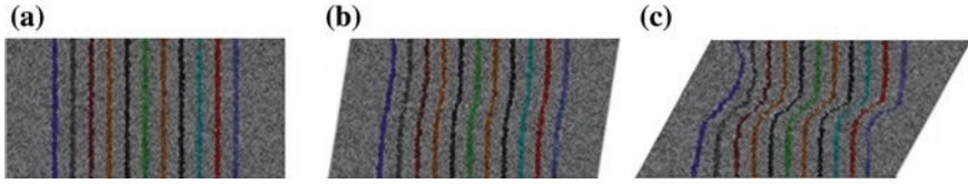
Fig. 2 Buckling of column of particles at different levels of shear strain. a \gamma_{xy}=0.0 . b \gamma_{xy}=0.12 . c \gamma_{xy}=0.50
