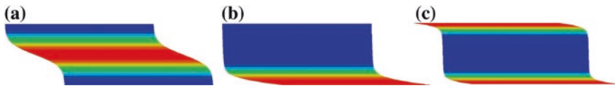
Fig. 5 Deformed shape of an infinite sand layer at residual state for: a Case I f_T = 0 and f_B = 0.0001 , b Case II f_T = 0 and f_B = 0.1 and c Case III f_T = f_B = 0.1
