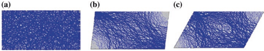
Fig. 3 Development of force chains at different levels of shear strain. a \gamma_{xy}=0.0 . b \gamma_{xy}=0.12 . c \gamma_{xy}=0.50
