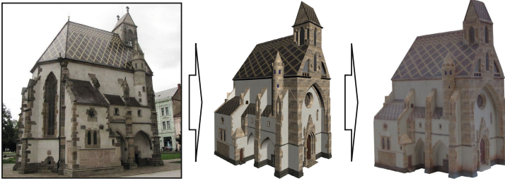
Fig. 3. Creation process of a tactile 3D model of St. Michael Chaple in Košice: real building (left), virtual 3D model created by SketchUp (middle), tactile 3D model printed by ZPrinter 450 (right)
