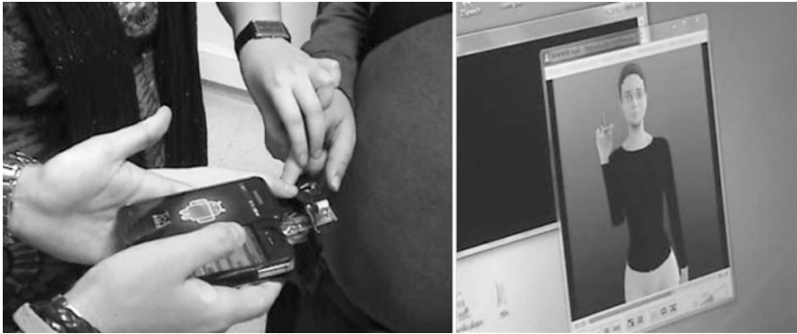
Fig. 3 Mobile phone, chip, and vibrator used for the translator tool and avatar shown on the computer
