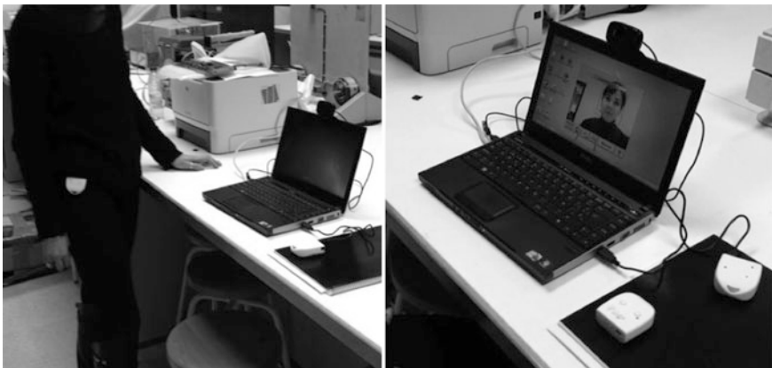
Fig. 2 User carrying a tag and tag located on the table to detect the RSSI signal
