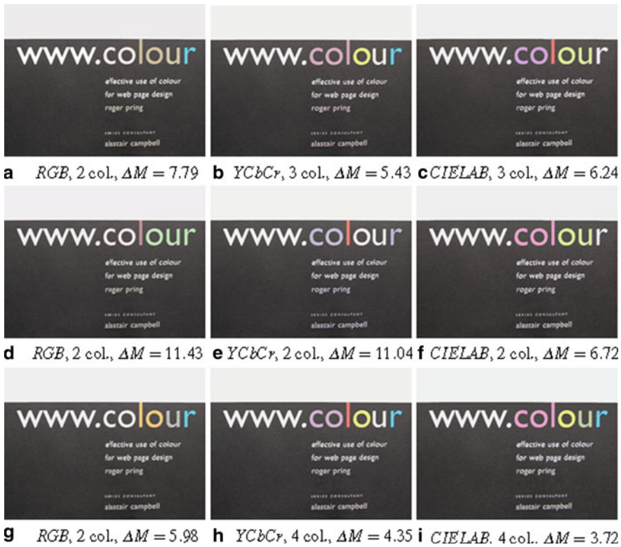
Fig. 12 KM results for the image from Fig. 9a, a, b, c results with DC initialisation, d, e, f results with SD initialisation, g, h, i results with MM initialisation ( k = 8 )
