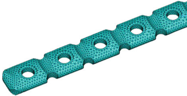
Fig. 7 Partial mesh of plate generated in Ansys
