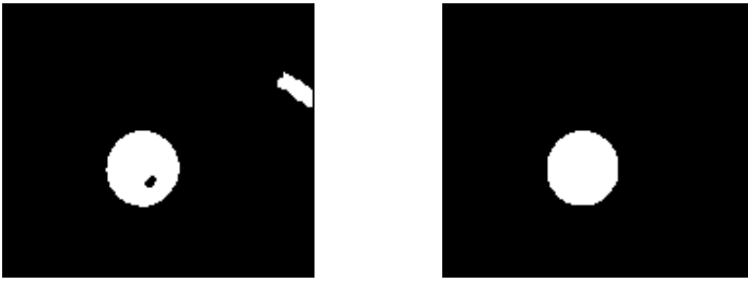
Fig. 4. Binarized version Wp of the watershed transform W , left, result of morphological operations and features extraction, right
