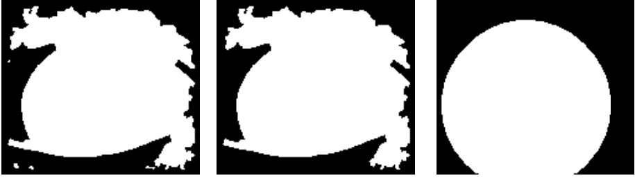
Fig. 6. Result after assignment to the background of the regions of W that are adjacent to the frame and are not adjacent to the pupil, left. Only the region with the largest area is taken as foreground in W_i , middle. Circular mask, right.
