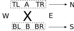
Fig. 2. Spatial regions around a mathematical symbol X. TL, A, TR, BL, B and BR denote top-left, above, top-right, bottom-left, below and bottom-right regions respectively. N – Northern region, S – Southern region, E – East, W – West.
