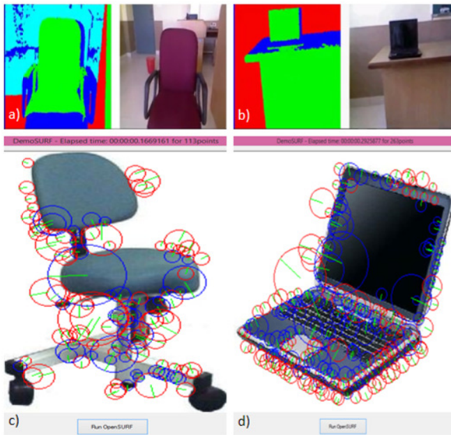
Fig. 3. a) Depth image of a chair acquired by Kinect b) Depth image of a RGB laptop on a table. Colors indicate distance ranging from safe to very close c) SURF interest points detected in a sample RGB chair image d) SURF interest points detected in a sample RGB laptop image.
