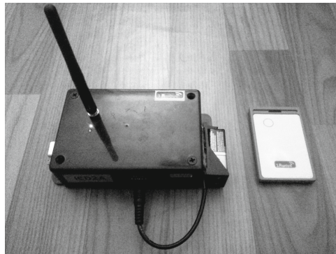
Fig. 2. RFID Reader (left) and Tag (right)
