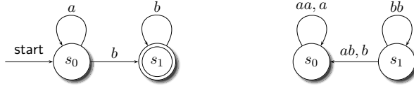
Fig. 1. A DFA accepting the language a^*b^+ (left), and its reverse DFA with lookahead two (right). The labels on the edges indicate the complete content of the input window (but only 1 symbol is “consumed”).
