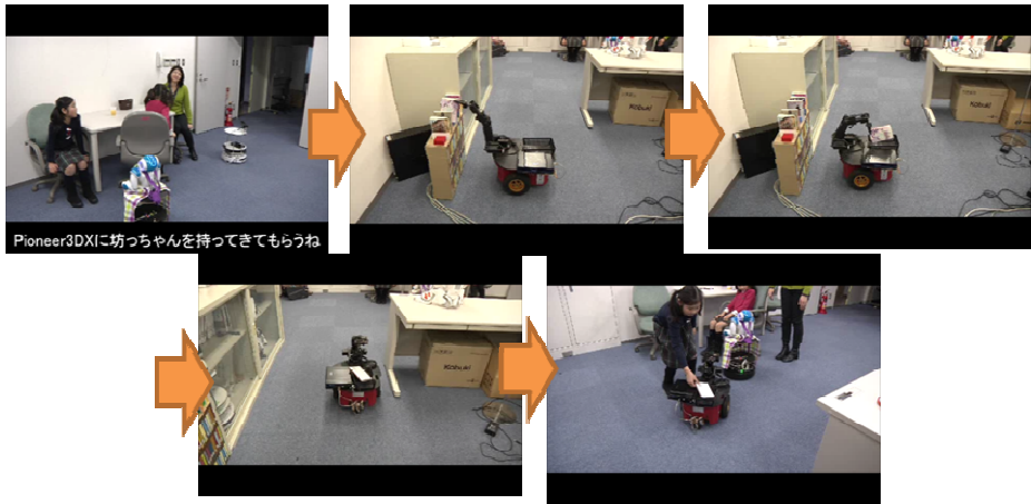
Fig. 11. As NaoTorso interacts with the user, Pioneer3DX carries the requested book to the user
