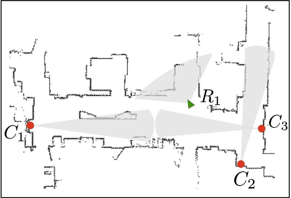
Fig. 4. Map of one corridor of the office with overlaid the position of three static cameras (red circles) and one mobile agent (green triangle) (Color figure online).
