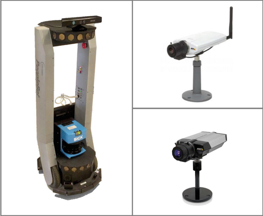
Fig. 5. The nodes of the network. On the left, the mobile agent PeopleBot. The robot is equipped with a laser range-finder SICK LMS200 and a Kinect. On the right, two different AXIS cameras: on the top, a Mpixel Axis IP color camera with 1280 \times 1024 . On the bottom, an Axis IP color cameras with a 640 \times 480 pixel camera.
