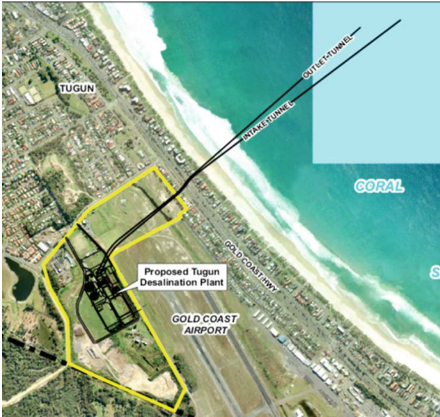
Fig. 3.11 Gold Coast SWRO plant location and schematic of intake and outfall tunnels
