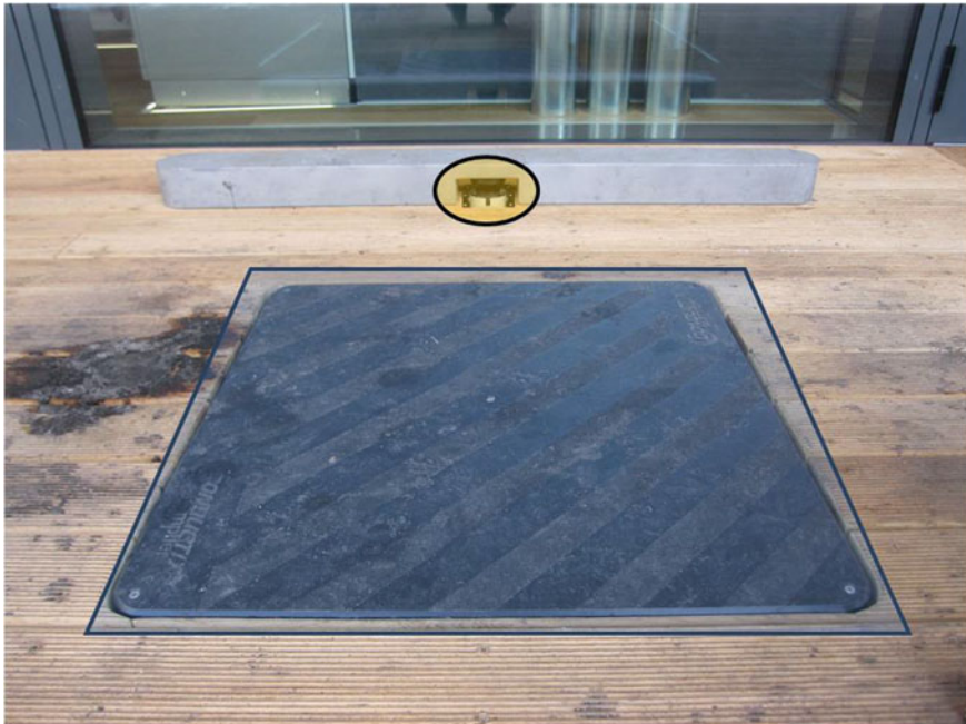
Fig. 6 Prototype inductive charging station for the usage in general public. The active power transfer zone (marked in blue ) is monitored by a LIDAR system (marked yellow ) (Photo by IAV) (color figure online)
