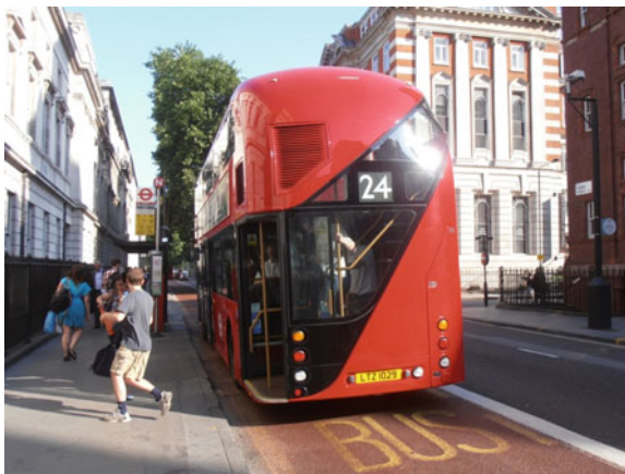
Fig. 1 The New Bus for London is powered by diesel-electric hybrid technology (photo S. Shaw)
