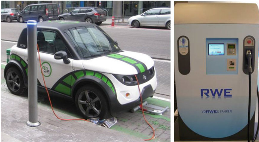
Fig. 1 Conductive charging of electric carsharing in Brussels and CHAdeMO charging station (Photos by IAV)
