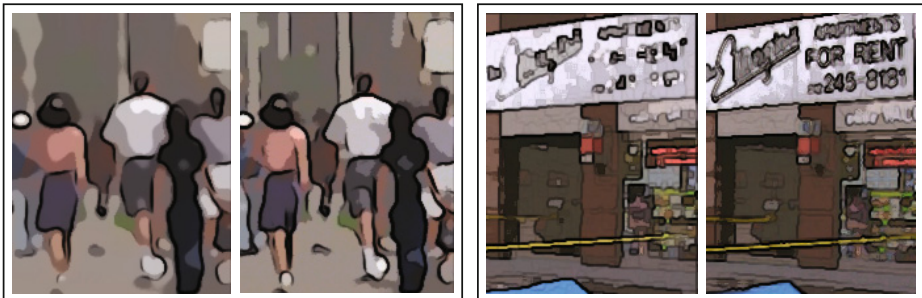
Fig. 4. Observations: Less than complete edge contouring on the color-quantized regions found by bilateral filter ( left pair ), and obvious loss of details using Kuwahara filter ( right pair ). The right-side image of each pair uses the proposed method.
