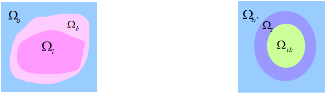
Fig. 3. Different regions in blending area. Fig. 4. Luminance contrast sampling. \Omega_{ib} \Omega_o(\alpha = 0) , \Omega_b(0 < \alpha < 1) , and \Omega_i(\alpha = 1) corresponds to regions ( \alpha > 0 ) including represents for the outer, border and inner both border and inner region in source and target image, \Omega_s is the luminance contrast sampling area.
