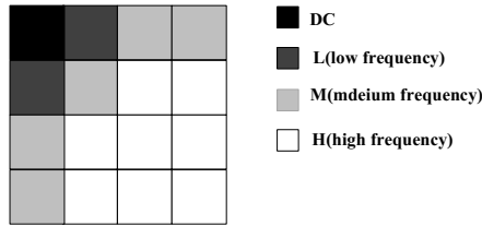
Fig. 1. Classification indicators for a 4 \times 4 DCT block
