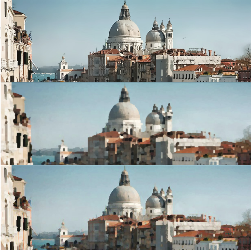
Fig. 3. Edge-preserving region smoothing using bilateral filter ( top ), Kuwahara filter ( middle ) and the proposed AD-SNN filter ( bottom ) on a photograph of the Grand Canal in Venice.
