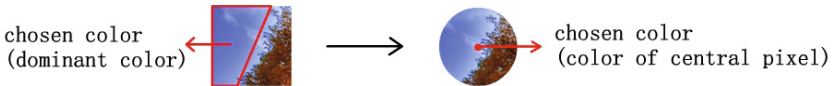
Fig. 2. Comparison of sampling technique and chosen color. (a) grid-sampling used in [9], and the dominant color determined by hue is selected as the chosen color. (b) circular region sampling used in our method, and the color of central pixel is selected as the chosen color.
