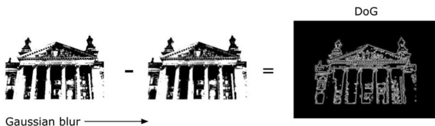
Fig. 6.12 Illustration of the difference of Gaussian's operator
