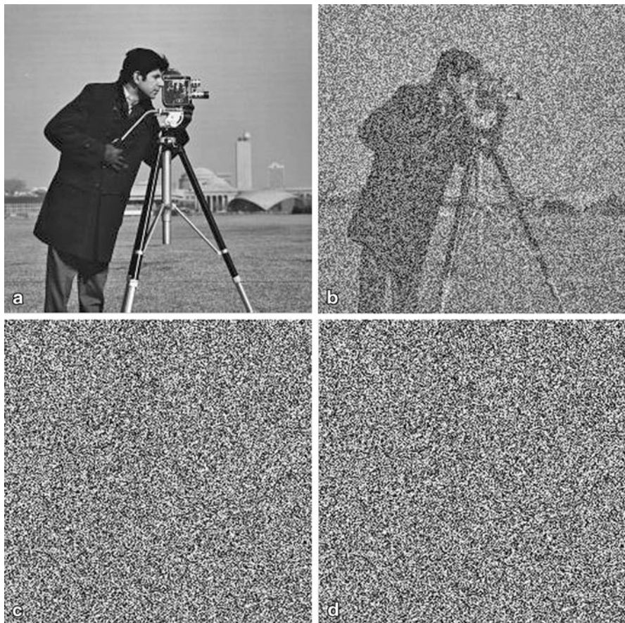
Fig. 1.15 Result of RPM-transformation. a Original image. b RPM-transformed version of the image shown in (a) : \beta = 1.5 . c RPM-transformed version of the image shown in (a) : \beta = 20 . d RPM-transformed version of the image shown in (a) : \beta = 50
