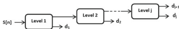
Fig. 2 The j th level TQWT based decomposition performed by iteratively applying two channel filter banks to the low-pass sub-band signals
