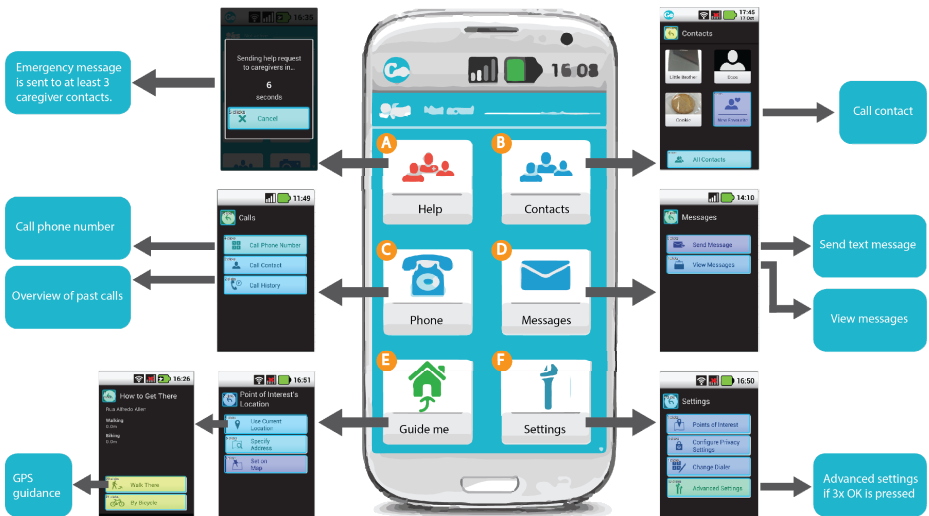
Fig. 1. The smartphone interface used for this study. The menu options are A) Help. B) Contacts. C) Phone/calling. D) Messages. E) Guide me home function and F) Settings.
