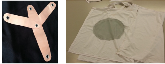
Fig. 2. (a) The PCB shape in a Kapton polyimide film, attached to fabric using Anorak snaps. (b) Double layer with mesh fabric to adjust the PCB in the Wrap top.
