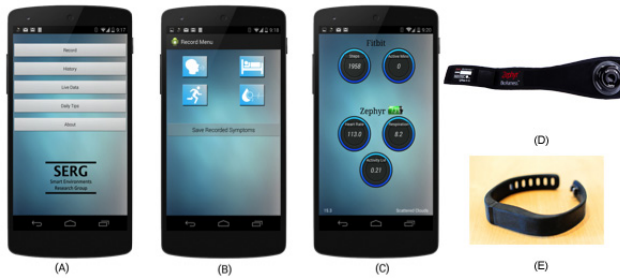
Fig. 2. Participant interface of the CAS monitor, (A) presents the main menu, (B) the manual recording selection screen and (C) the method of displaying live data from the sensors to participants. (D) Presents Zephyr Bioharness chest strap ( http://zephyranywhere.com/ ) and (E) presents the Fitbit Flex wrist strap ( http://www.fitbit.com/uk/flex ).
