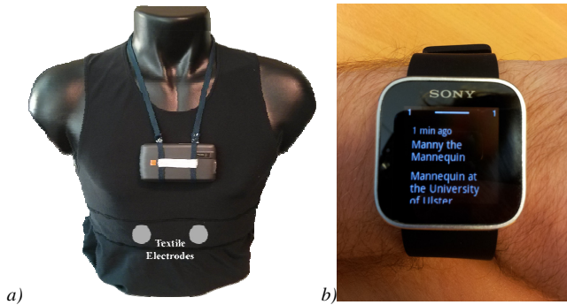
Fig. 2. miLifeCam technology components worn by the participants during the evaluation. a) ZTE Blade smartphone on a lanyard and b) Sony Smartwatch.
