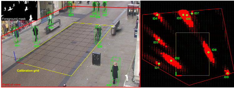
Fig. 2. Detection of 3D persons using the perspective grid (left) and an example top view of the grid (right)
