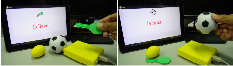
Fig. 5. Functional System: a key and a ball are recognized by the system and the respective cards are created and sent to the tablets
