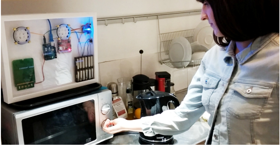
Fig. 2. A Powerchord prototype in use, monitoring a microwave oven and kettle
