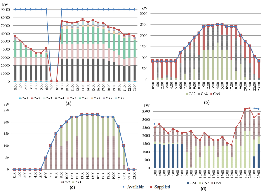
Fig. 1. Power supplied (red line) and available (blue line) by FAi to CAj. (a) Power supplied by FA1-5 to CA1-9. (b) Power supplied by FA8 to CA7-9. (c) Power supplied by FA9 to CA2-3. (d) Power supplied by FA10 to CA1, CA7 and CA9.
