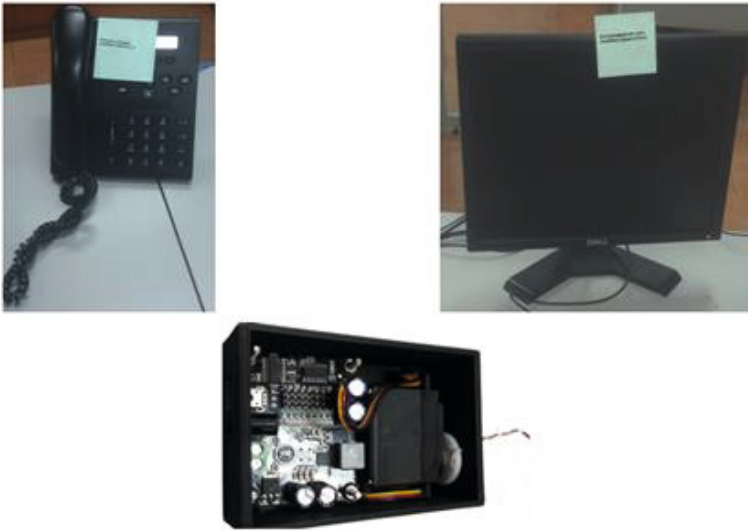
Fig. 2. Notifications shown in context for two different documents and the case with Phidgets that contains the servo that moves the pos-it note (appear and disappear)
