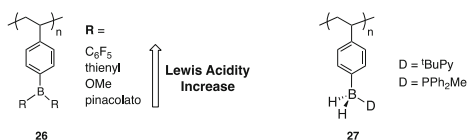
Fig. 3 Lewis acidity tuning of organoborane polymers
