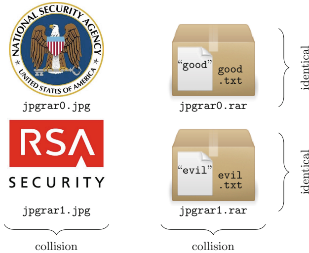
Fig. 2. Colliding JPEG/RAR polyglot file pair for malicious SHA-1 (cf. Table 4).
