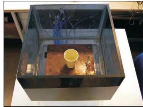
Fig. 3 Imaging setup. A plastic cup of vegetable oil is put at the center of the antenna array.
