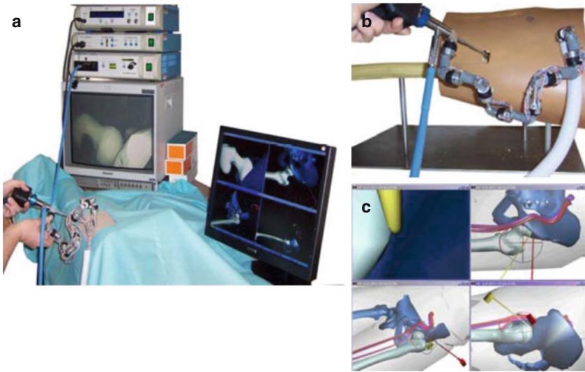
Fig. 3.3 Computer-Aided arthroscopic hip surgery system from Gunay et al. [34]. (a) Setup of complete computer-aided system. (b) Encoder linkage tracks an arthroscopic camera applied to a hip joint model. (c) Snapshot of computer display which shows the surgical tools and patient anatomy from multiple angles. Reproduced from Monahan et al. [33] with permission from IOS Press.
