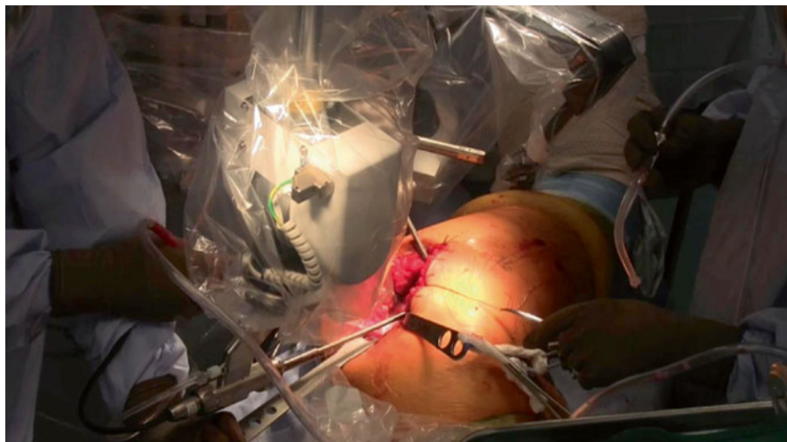
Fig. 16.4 ROBODOC preparing the femoral canal during THA
