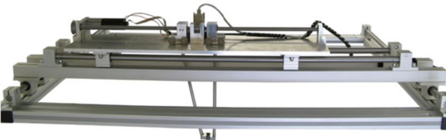
Fig. 20.2 Three degrees-of-freedom mechanism capable of applying a pure axial mechanical load to the patient’s cervical spine (Reproduced from Elias de Oliveira [15] with permission)
