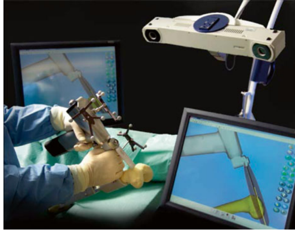
Fig. 9.6 Navigated Freehand Cutting system, early elementary prototype used on Study1
