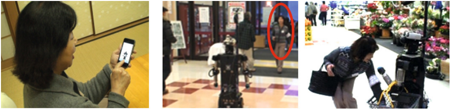
Fig. 27. An example of personalized service : (a) requesting a robot from her mobile phone, (b) detecting the customer's arrival, and (c) shopping with the customer
