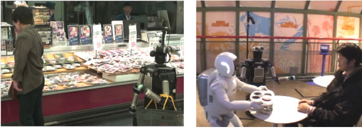
Fig. 2. Example scenes using our Network Robot System framework. (a) helping a customer with shopping, (b) collaboration between heterogeneous robots.
