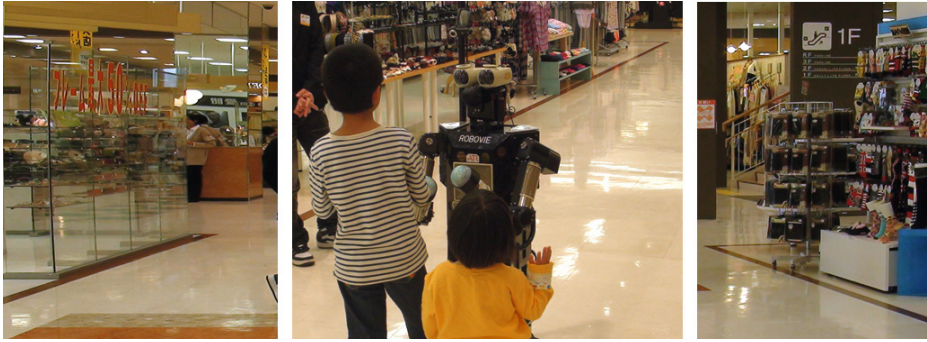
Fig. 19. Dangerous areas in a shopping mall. Left: glass walls. Center: movable tables and shelves where only legs are visible to ground-level LRF's. Right: movable clothing rack where only the center pole is visible to ground-level LRF's.
