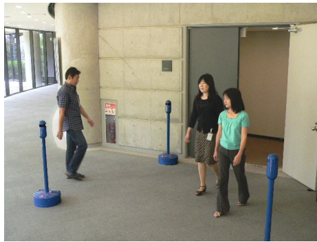
Fig. 3. The ATRacker system features Hokuyo laser range finders mounted on portable poles which can easily be placed in public spaces
