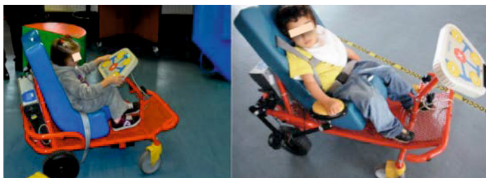
Fig. 2. Two children driving the PALMIBER vehicle with different interfaces (console of directions and single switch)
