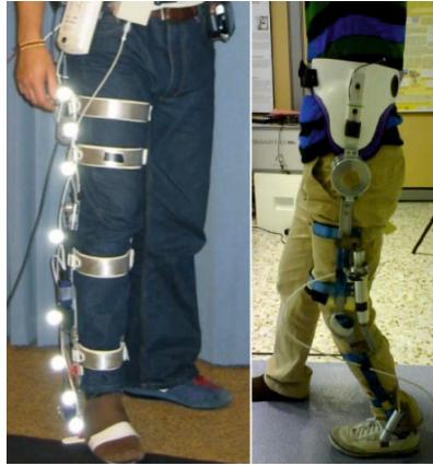
Fig. 1. Example of an exoskeleton robot: lower limb orthotic exoskeletons
