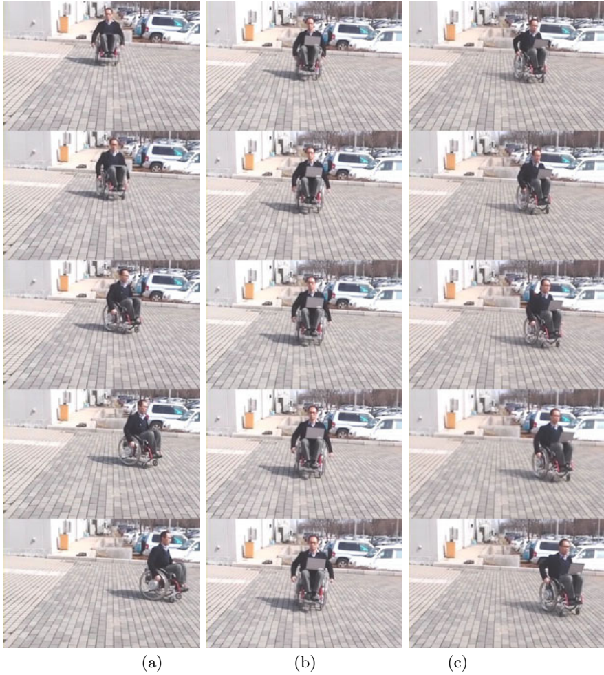
Fig. 29. Outdoor experiments on a sidehill: (a) without rotational disturbance rejection control (b) with rotational disturbance control (c) driving the wheelchair downhill diagonally with the control
