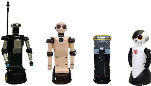
Fig. 24. Robots used in these studies, left to right: Robovie II, Robovie IIs, shopping-cart robot, Robovie-R3
