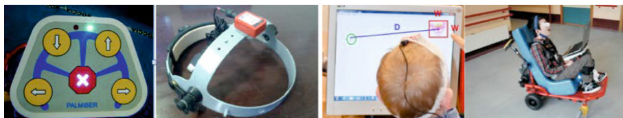
Fig. 4. Interfaces for driving the vehicle: console of direction, ENLAZA, an inertial head-mounted interface for driving the vehicle and control the computer
