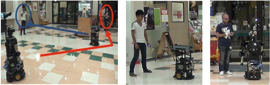
Fig. 20. Coordinating multiple robots: (a) Robots are given non-conflicting paths to reach their respective customers, (b) Each robot provides its service
