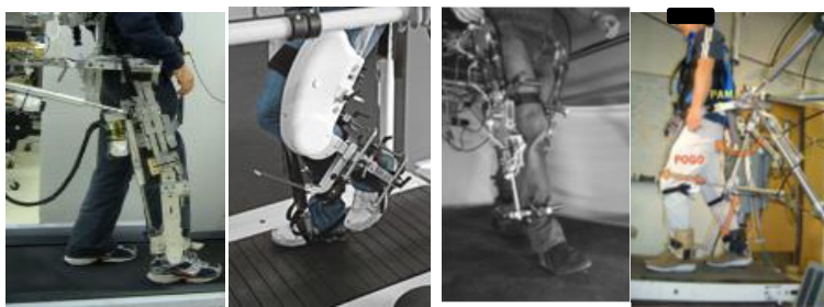
Fig. 11. Robotic orthosis of treadmill-based systems, from left to right, ALEX [58], Lokomat [59], LOPES [60], and POGO [61]
