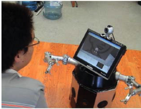
Fig. 15. Sobot User Interaction through Mobot, the Sobot has downloaded itself onto Mybot to enable monitoring of the user and thus providing anyplace and anytime service
