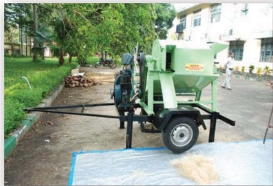
Fig. 13.1 Mobile coir fibre extraction machine
