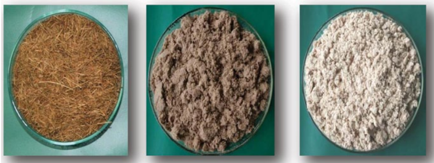
Fig. 13.8 Tender coconut fibre after organosolv pulping and bleaching. (Sarma and Ravindranath 2006a, b)
