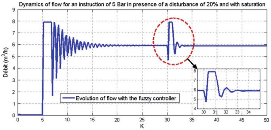
Fig. 27 Evolution of flow with the Fuzzy controller with saturation
