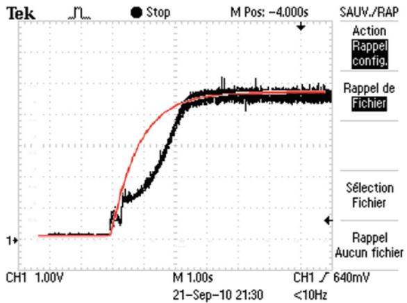
A comparison was made between the estimated outputs and actual outputs collected using a digital oscilloscope (Figs. 15 and 16).
