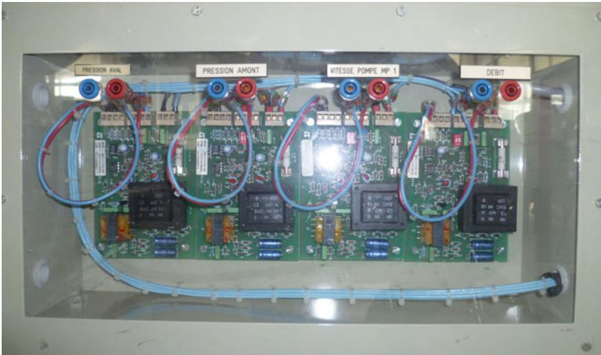
Fig. 8 Connectors of sampling signals (pressure and flow)
