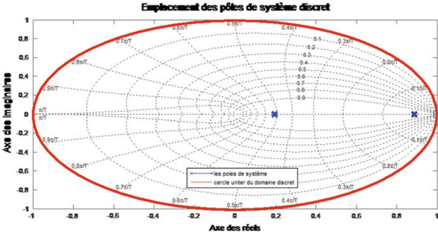
Fig. 18 Location of discrete time system poles
