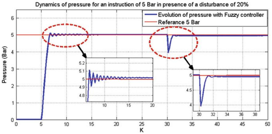
Fig. 25 Evolution of pressure with the Fuzzy controller
