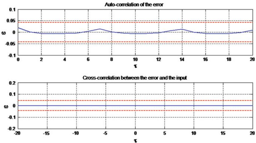
Fig. 13 Validation results autocorrelation and cross-correlation of pressure output
