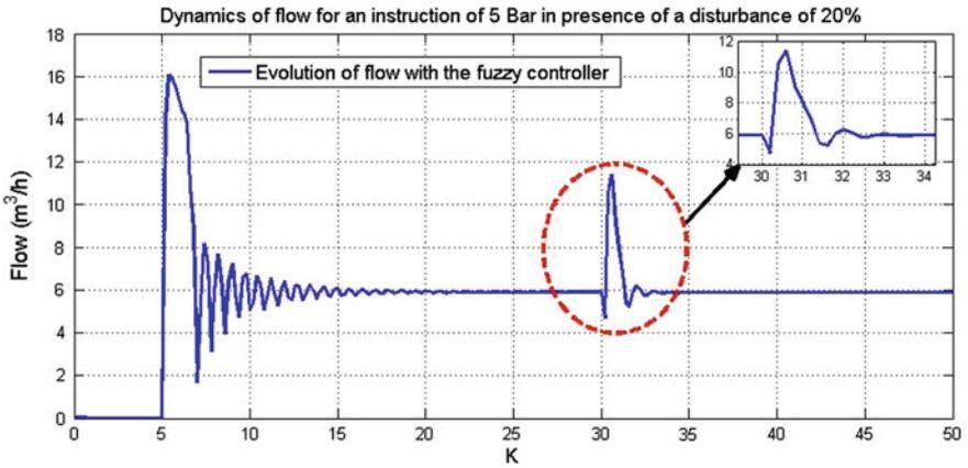
Fig. 26 Evolution of flow with the Fuzzy controller
