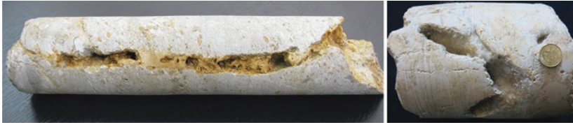
Fig. 3.15 Secondary porosity, but restricted: cavities partly filled with recrystallized calcite in limestone core samples
