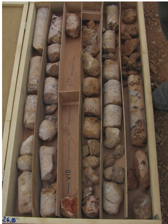
Fig. 3.21 Core samples taken from the exploratory borehole at Ourkiss dam site (Oum el Bouaghi, Algeria). Great variation in lithology of Turonian limestones: fissuration degree, texture, and impurity. No sample taken from a section of around 1 m in length indicates the presence of a cavern
