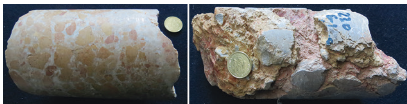
Fig. 3.13 Carbonate breccia: well cemented and compact with very small porosity ( left ) and poorly cemented ( right )
