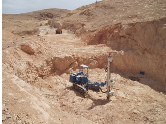
Fig. 11.8 A small drilling rig used for drilling test holes in upper Cretaceous limestones at Ourkiss dam site (North Algeria)
