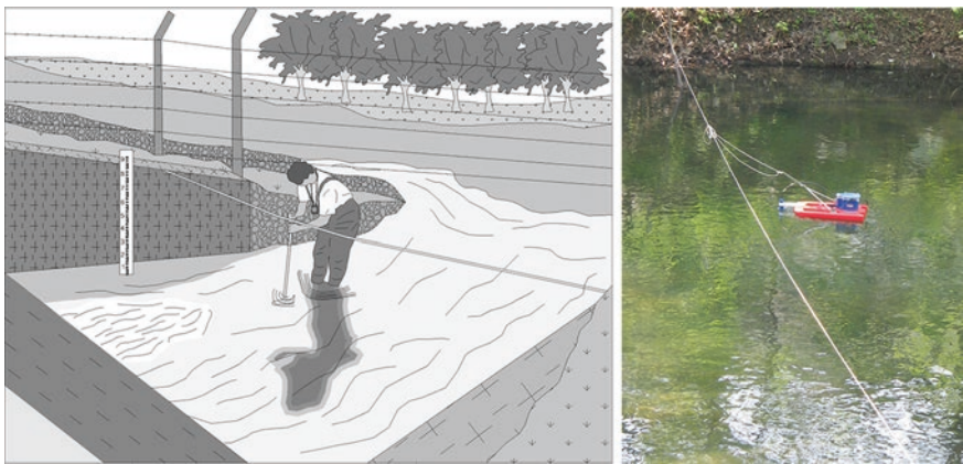
Fig. 6.5 Classical hydrometry with current meter ( left ) and Doppler radar for depth/velocity scanning ( right )
