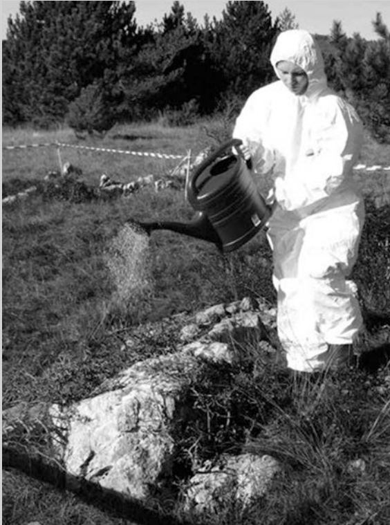
Fig. 17.12 Validation of vulnerability results by execution of an artificial tracer test. By spreading a tracer on the land surface, a simulation of contamination can be done. By monitoring of the tracer appearance at the spring(s), the level of “contamination” can be achieved
