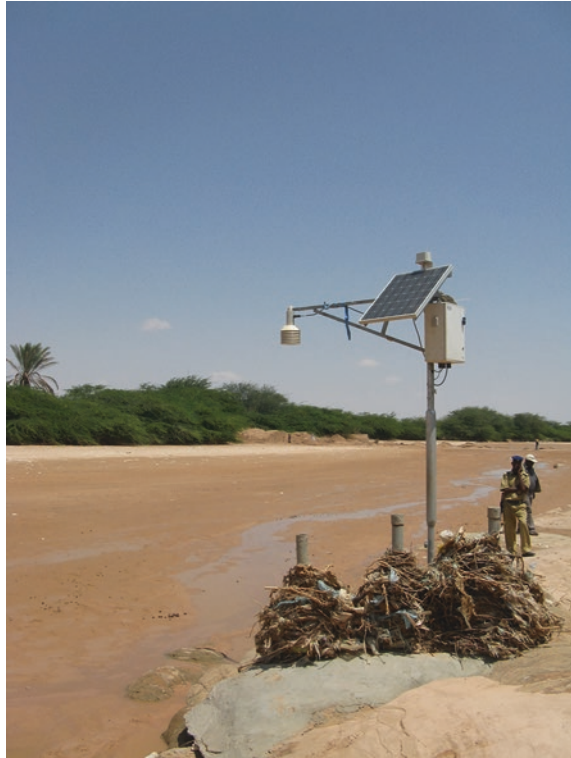
Fig. 6.6 Gauging station and data transmitter on wadi (temporary stream) bank near Hargeysa in northern Somalia
