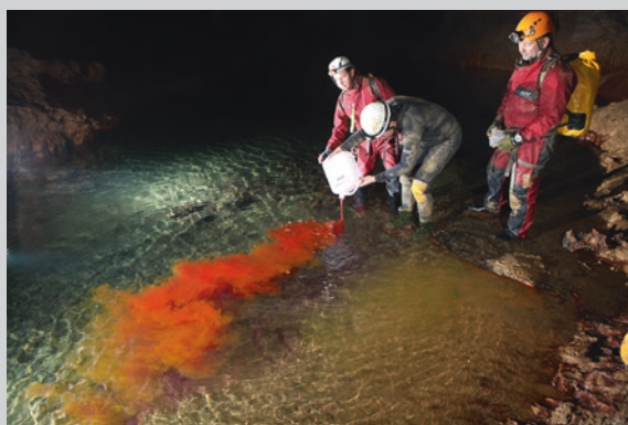
Fig. 4.8 Tracer injection into Blauhöhle cave, Germany (photo courtesy of A. Kücha). The tracer powder was transported to this hard-to-reach injection site in a plastic canister, mixed with water from the cave stream, and directly released into flowing water to ensure optimal tracer transport. In-cave dye tracing makes it possible to obtain spatially resolved information on conduit flow (Lauber et al. 2014)
