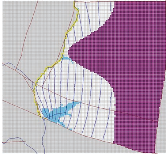
Fig. 10.12 Flow solution for the EPM model. Groundwater flows toward the intermittent stream and the spring. The purple cells indicate dry cells in the top layer at the low-permeable core of the anticline. Blue cells indicate flooded areas where the calculated potentiometric surface is above the ground surface elevation
