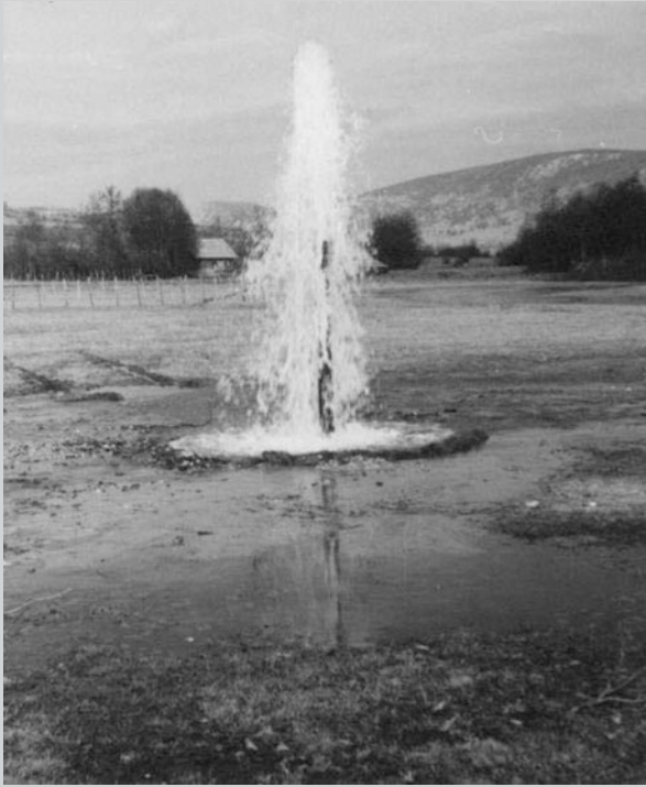
Fig. 16.22 Artesian flow from exploration well BM-159, limestones in the background (Courtesy of Mićko Radulović)
