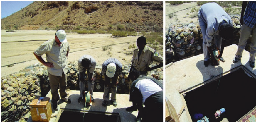
Fig. 12.7 Using groundwater dip meter for groundwater monitoring in Berbera (Somalia), see Box 12.1
