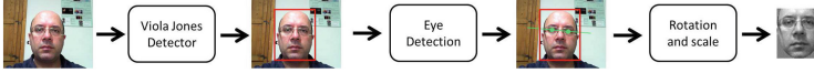
Fig. 2. Face detection and normalization: A Viola-Jones face detector detect the faces present in an image. When the face is well located in the space an eye detection is used to rotate and scale the face in such a manner that all face present the same scale and orientation
