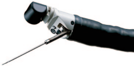
FIG. 2.2. Echoendoscope with linear transducer. (Olympus GF-UC140P, Olympus America, Center Valley, PA)
