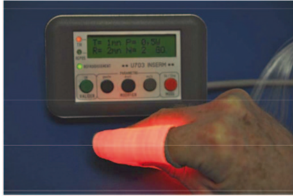
Fig. 3.2 Example of a textile based light delivery device that facilitates illumination of curved surfaces. (Reprinted with permission from Cochrane C, et al. [35])
