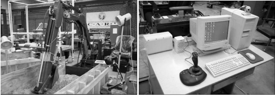
Fig. 2.3 Turn of the century NCSU experimental virtual laboratory featuring remotely manipulated teaching and research backhoe (Civil Engineering, Computer Science)
