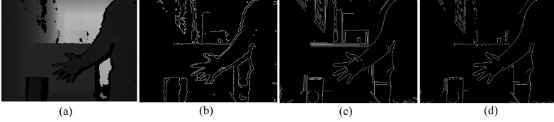
Fig. 2. (a) original depth map, (b) depth map discontinuity map, (c) initial depth discontinuity map, (d) refined depth discontinuity map
