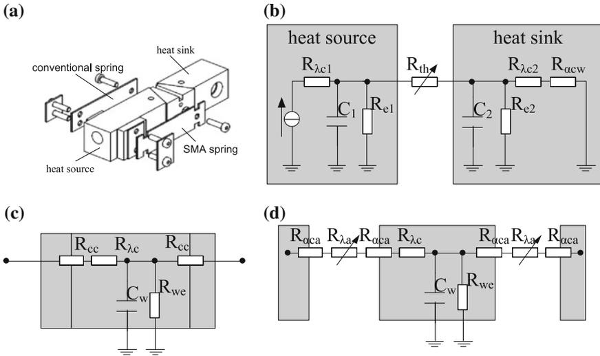
**Fig. 17.5** Experimental setup of the heat bridge and thermal equivalent circuits. **a** Overview on overall setup. **b** Network of overall setup. **c** Network for closed heat bridge. **d** Network for opened heat bridge
