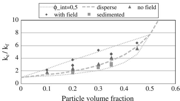
**Fig. 17.7** Thermal conductivity as a function of the particle volume fraction, related to thermal conductivity of the basic fluid. Theoretical (*dashed curve* for disperse case, *dotted curves* for magnetic field influence and deposited fluid at an internal volumetric fraction of 0.5) and measured values (*check marks*) for thermal conductivity, scaled to the basic fluid's thermal conductivity
