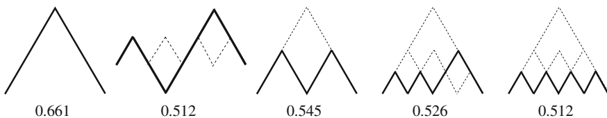
Fig. 1 Five displayed curves ( solid lines ) have different linearities measured by \mathcal{L}(C) . The straightness index has the same value for all five curves
