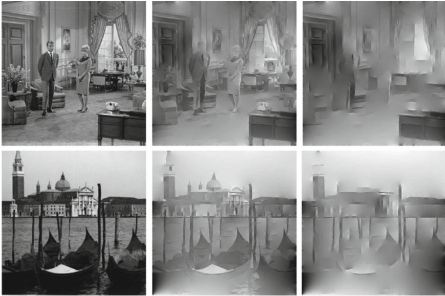
Fig. 8 Reconstructing the image from its filtered edges. ( left column ) original intensity image; ( middle column ) image reconstructed using all connected edges (minimum length: 25 pixels); ( right column ) image reconstructed using sections of curve with \mathcal{L}(C) > 0.95
